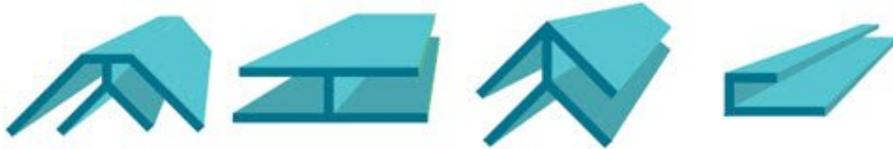
Apart from using trims (pictured above), both internal and external corners can be neatly done by bending the panels - just carefully cut the back face of the board along where the corner will be and shape the panel into the internal or external curve.
